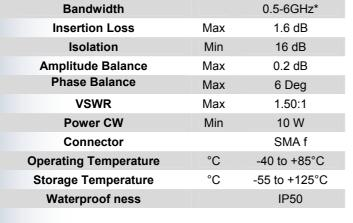
\* This power divider operates down to 300MHz with the guaranteed specs (see above), except: Isolation: 14dB min on range 300-500MHz VSWR input : 2.3 :1 max on range 300-500MHz
